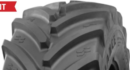
State-of-the-art materials and steel construction allow IF (increased flexion) radial tractor tires to deliver outstanding performance in any conditions. IF tires carry up to 20% more load at the same inflation pressure as conventional radials, or require 20% lower inflation pressure for the same load, to reduce soil compaction. (TUBELESS - STEEL BELTED - STUBBLE GUARD)
