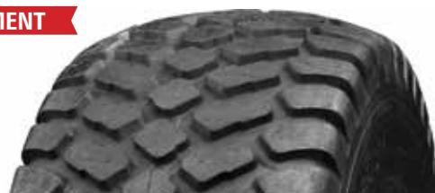
Steel-belted tire for both on and off road applications. Shoulder lugs provides better grip in muddy fields as well as in other soil conditions. Strong bead bundle with extra-thick reinforced sidewalls and high turn-up plies ensure excellent stability and protection against external damages. (TUBELESS - STEEL BELTED)
