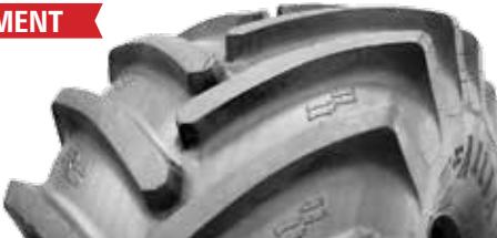
Modern continuous-angle lug ensures smooth roading and superb traction. Steel-belted construction coupled with stubble-resistant compound makes the tire exceedingly resistant to punctures and damage from today's hybrid crops. (TUBELESS - STEEL BELTED - STUBBLE GUARD)
