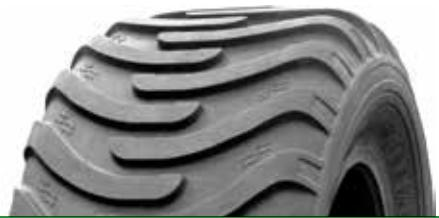
Radial flotation tires designed for minimal soil compaction and maximum tire life. For agricultural applications, primarily used on spreaders and special trailers (i.e. sugar cane production). Flat footprint, steel belts, rounded shoulders and low inflation pressure for superior performance over bias flotation. (TUBELESS - STEEL BELTED)
