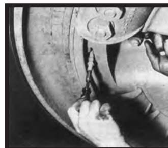
Removing valve core from single piece wheel.
